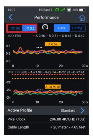
The HDBaseT Performance overview gives the user a live overview of the signal passing through the MS-TestPro for both MAX ERR and MSE ERR on both Transmitter and Receiver modules. The tester can be switched between TX and RX by using the selection switch at the top of the screen as highlighted above.
