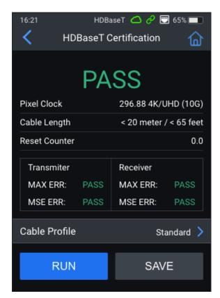
Once the test has finished, a PASS or FAIL result will be shown on the tester screen. For more information on MAX ERR and MSE ERR values, see next page.
