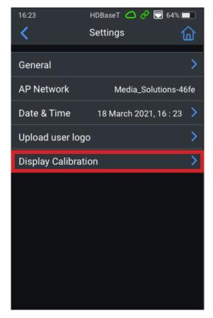
Follow the instructions on screen, pressing the tip of the stylus on the red cross-hairs at the given points on the screen. Once a calibration point has been confirmed, it will turn white, and a new cross-hair will appear. A count-down timer will appear in the centre of the screen between presses. Please complete the stylus press within the countdown period.
