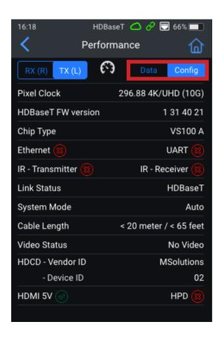
The 'Config' data page shows the capabilities of the HDBaseT chipsets in use on both TX and RX side (using the switch in the top left of the screen).
