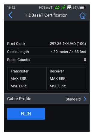
If using a CATx cable that has been included into the pre-defined Cable Profiles of the MS-TestPro, use the Cable Profile selection towards the bototm of the screen to select the cable type being used. Otherwise, leave this as 'Standard'.
