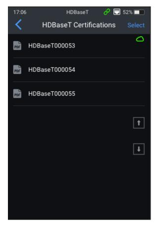
All reports from any of the tests that the MS-TestPro can carry out will be saved into this location for download onto a USB stick inserted to one of the 4 slots on the top of the MS-TestPro.
