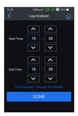
The Log Analyzer creates 2x .csv file download documents. One document relates to the testing data for the Transmitter module, the other for the Receiver module.
