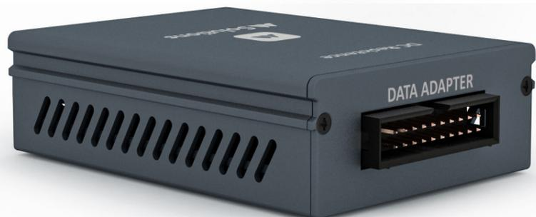
DC Resistance provides a deeper analysis of the infrastructure cabling quality, analyzing each twisted pair. It provides an inner look on the CATx wiring quality and its ability to support a high quality HDBaseT/Ethernet transmission while supplying PoE / PoH with high efficiency.
